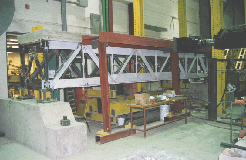
Figure 4 27-foot long deck-truss model in retrofitted condition and pseudo-dynamic test set-up at the University of Ottawa
